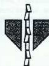
INCORRECT Insufficient support for blade.
