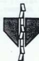
CORRECT Maximum support for blade.
